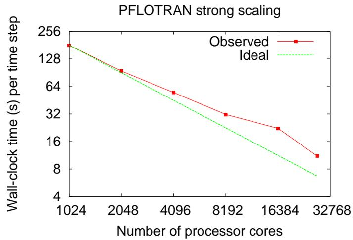
Figure 2: Strong-scaling performance on the Cray XT4 of the computation phase (no I/O) of PFLOTTRAN for a variably-saturated flow problem with 270 million total degrees of freedom.
