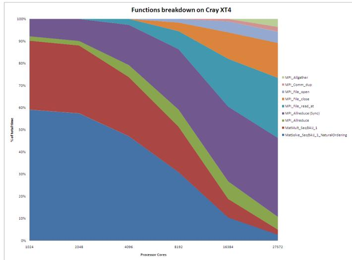
Figure 11: Breakdown of contributions of different routines to overall execution time of the 270 million degrees of freedom flow problem run on the Cray XT5 for 30 time steps, with no disk output.
