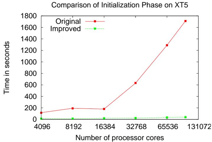
Figure 10: Performance comparison of the original and improved initialization routines on the 270 million degrees of freedom flow problem on the Cray XT5. The curve labeled “original” depicts the performance when all processes open and read from the HDF5 file, and the “improved” curve depicts performance when only a subset of processes read the data and then broadcast to the other members of their I/O group.
