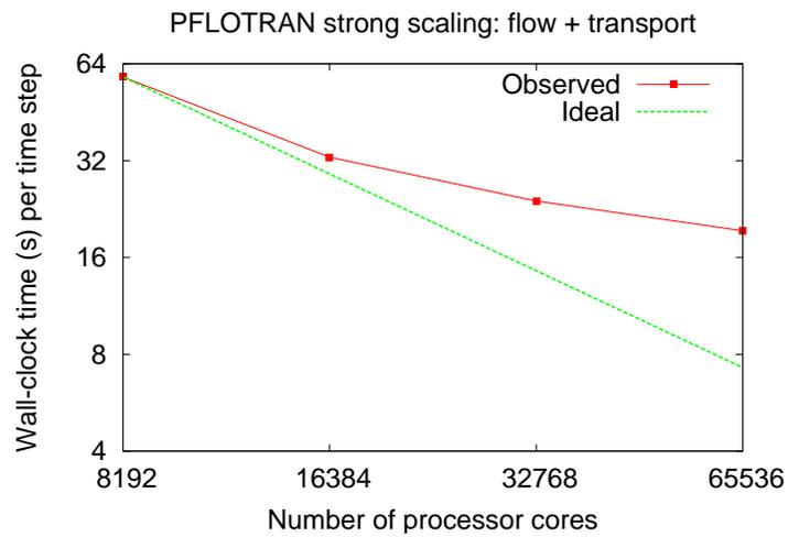
Figure 7: Combined strong-scaling performance of flow and transport solves for a coupled flow and reactive transport simulation on an  $850 \times 1000 \times 160$  cell grid with 15 chemical components.
