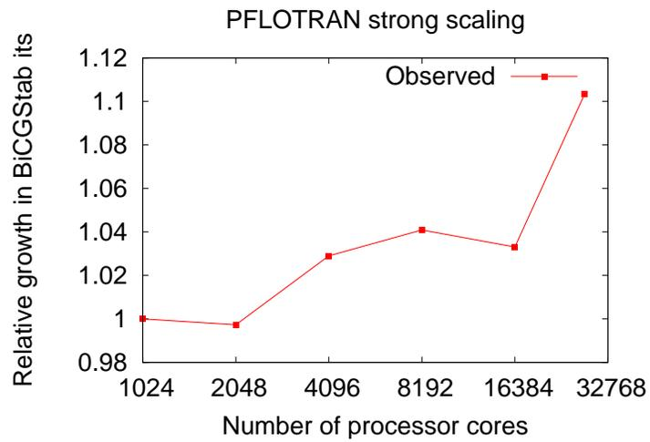
Figure 3: Growth of BiCGstab iterations for the strong-scaling case depicted in Figure 2.
