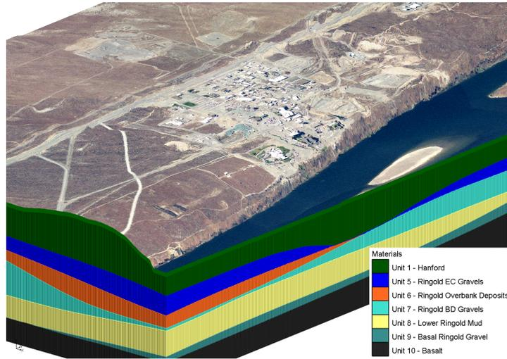
Figure 1: Hanford 300 Area stratigraphy ( $z$  scale = 20x,  $z$  axis ranges 70–130 meters).
